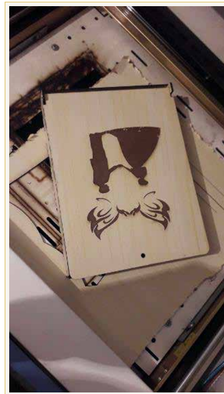
Figure 5.3: The product customized for the wedding occasion after being produced on the laser machine, and the details of the wooden cutting and engraving
