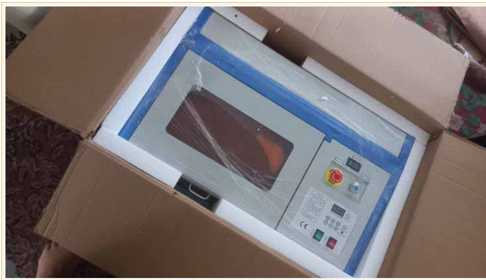
Figure 5.1: The laser machine (CO2)
