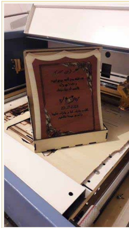
Figure 5.3: The product customized for the wedding occasion after being produced on the laser machine, and the details of the wooden cutting and engraving
