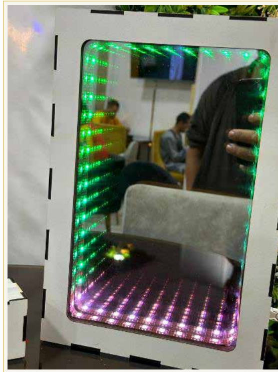
Figure 5.6: A sample of the illuminated mirror with a three-dimensional effect (Infinity Mirror)
