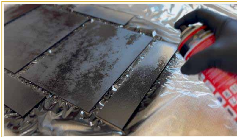
Figure 4.2: The stage of spraying the wooden pieces with the matte black paint (Matte Black).
